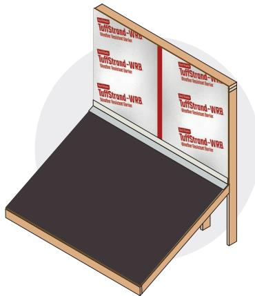
Measure and cut IBC-approved adhesive flashing width at least 12". Install 6" of flashing to TuffStrand on wall and 6" of flashing to roofing underlayment.
